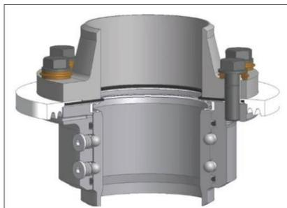
Figura 5-7- Insulating flange
